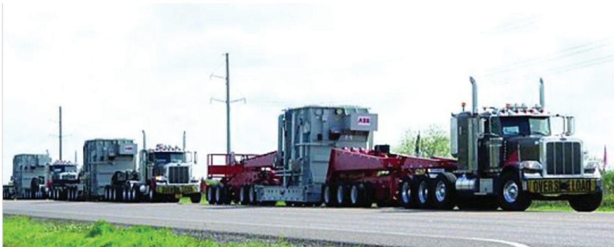
FIGURE 6.3 Three ABB single-phase 345 kV compact replacement transformers being moved from St. Louis, Missouri, to a substation in Houston, Texas, under a Department of Homeland Security demonstration project. SOURCE: DHS (2012).
