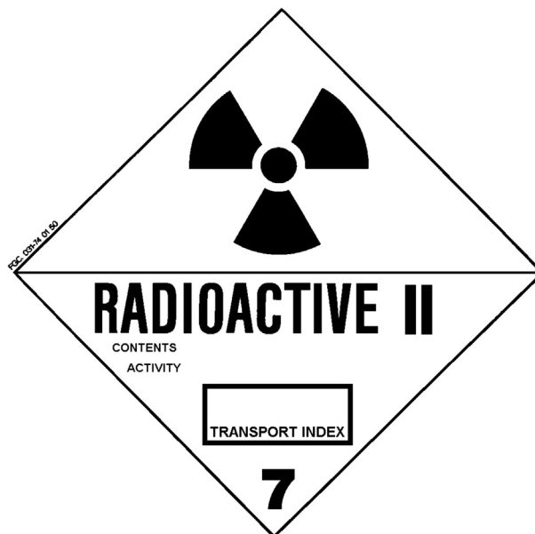
Figure 15.15 Label for shipment of radioactive material of class II. "II" in red with a yellow background.
