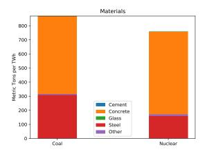
Figure 7.4: Concrete and steel, coal versus nuclear.[128][Table 10.4]
