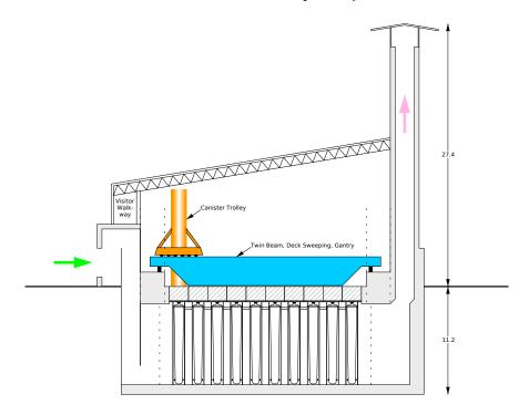
Figure 2.11: Section of Vault
