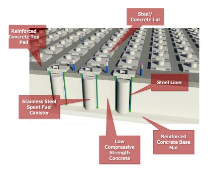
Figure 2.7: Cutaway view of the storage system
