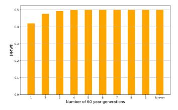
Figure 2.5: Hi-Store Unit Cost as a function of storage time
