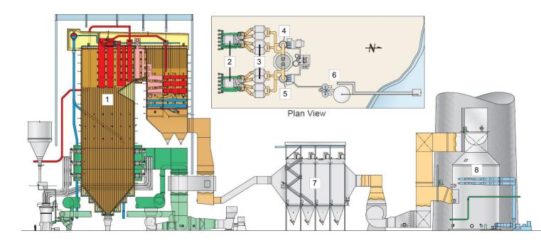
Figure 7.3: 660 MW Tanjung Jati boiler and gas handling equipment. 1. Furnace, 2. boiler house, 3,7. Electrostatic Precipitators (modern baghouse), 4,5,8 scrubbers, 6. wet scrubber limestone silo
