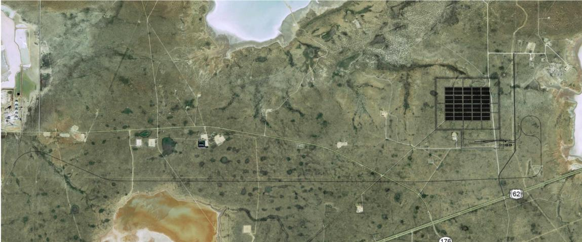
Figure 2.9: Satellite view of the Hi-Store facility. If the US were to go all nuclear, the 20 pads on the right would handle at least 12 years worth of used fuel.
