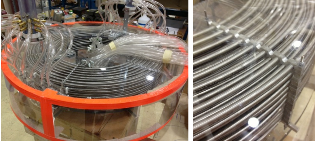
Figure 3-7. UCB CTAH test bundle (left) with close up of tube support bars (right).
