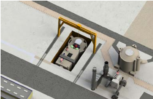
(C) Below-grade structures installed as six structural modules and reactor cavity module
