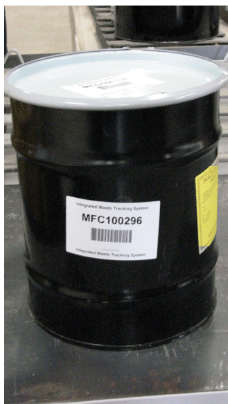
Figure 1. 10-gal container containing poly bottle with 2-3 ounces of NaK.
