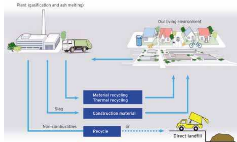
Figure 7.8 - Overall solid waste treatment and recycling scheme for a community using the gasification and ash-melting process
