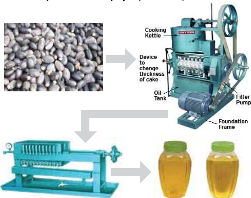
Figure 3.1 - Processing of jatropha seeds to produce oil
