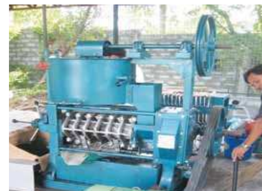
An Indian-made mechanical oil extractor (front) with a plate-and-frame filter press (behind the oil extractor, partly hidden) located at the jatropha oil pilot plant owned by Philippine Forest Corporation. (Photo by LAUDS Technologies, Inc., 2007).
