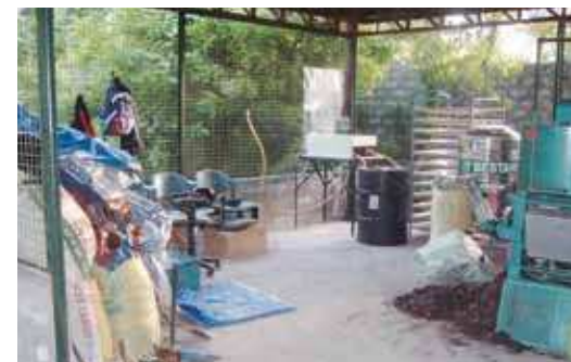
A pilot plant for the production of jatropha microemulsified hybrid fuel comprising a mechanical extractor (green colored equipment on the right) and a small MHF machine (silver colored equipment on the center) located at Philippine Forest Corporation. (Photo by LAUDS Technologies, Inc., 2007).
