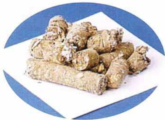
Figure 7.2 - Refuse-derived fuel produced in a modern RDF plant
