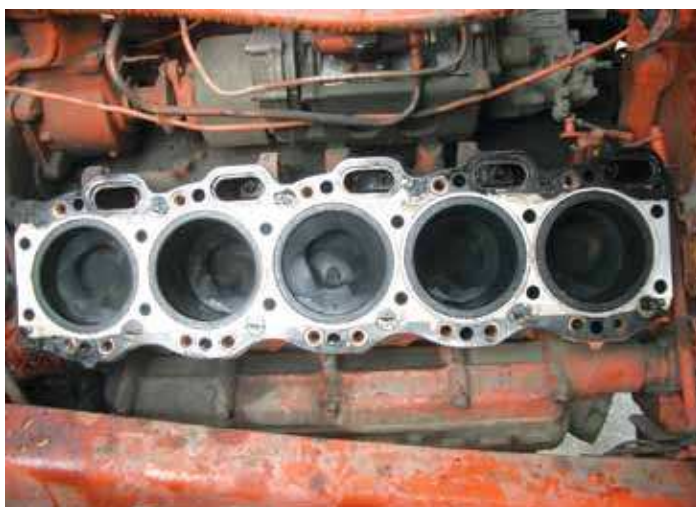
View of open truck engine cylinder. (Photo by Nippon Ecosolutions, Ltd. and LAUDS Technologies, Inc.)
