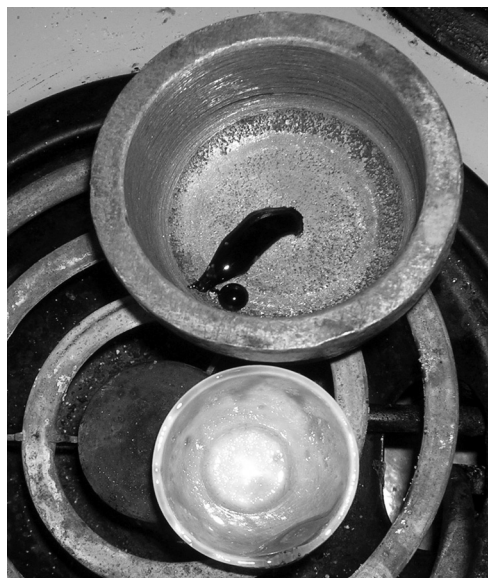
Fig. 8. Mortar, crucible, and glass sample.
