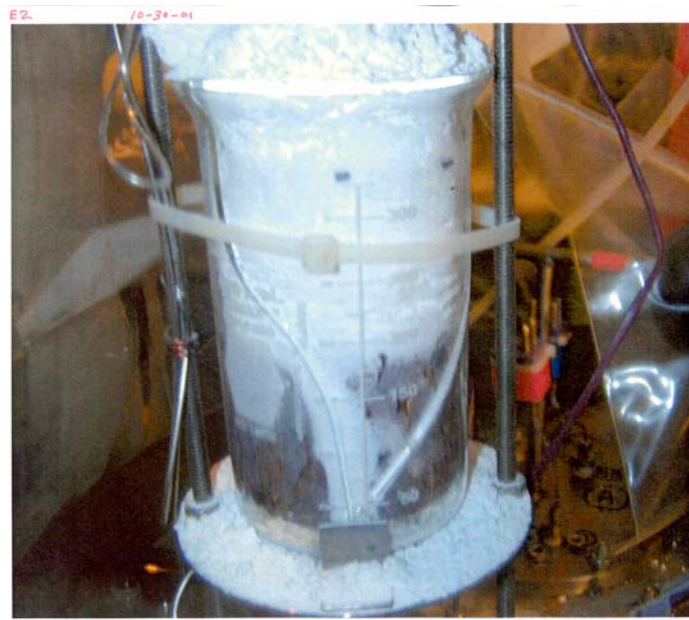
Figure 14. Sample E2 after 123 days exposure.
