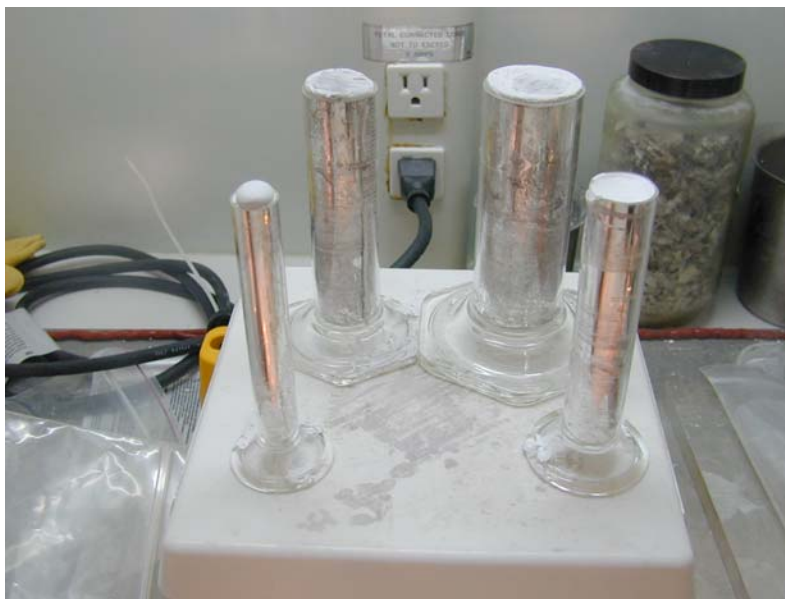
Figure 6. Kimex ® graduated cylinders filled with sodium.
