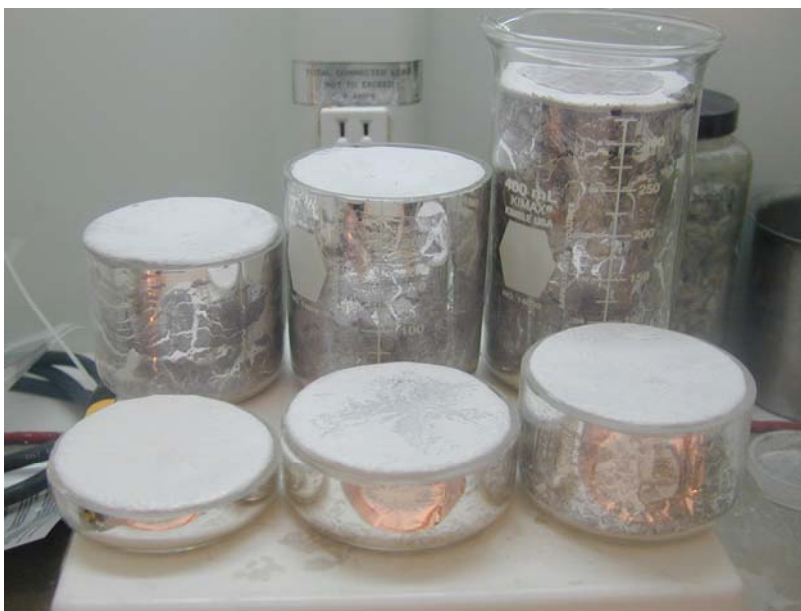
Figure 5. Kimex ® beakers of various heights with metallic sodium. The white layer is sodium oxide.
