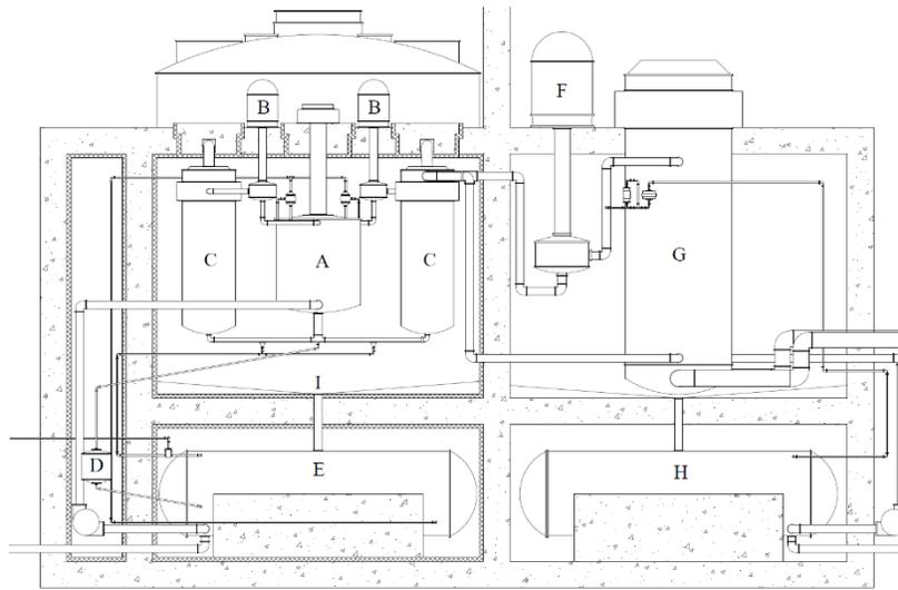
**Figure 2.** Simplified reactor schematic, depicting the primary loop, intermediate loop, drain tank, and outlet to the fission gas processing system. Figure legend: A) reactor vessel, B) fuel salt pumps, C) primary heat exchangers, D) freeze valve, E) primary loop drain tank, F) intermediate loop salt pump, G) steam generator, H) intermediate loop drain tank, and I) fuel catch basin.
