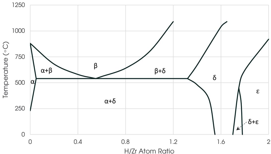
**Figure A.1.** Zr-H phase diagram, adapted from [31].
