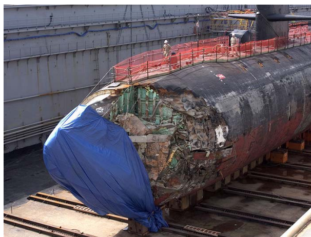
Figure 128: Los Angeles-class Fast-Attack Submarine USS San Francisco (SSN 711) in Dry Dock to Assess Damage Sustained after Running Aground 350 Miles South of Guam
