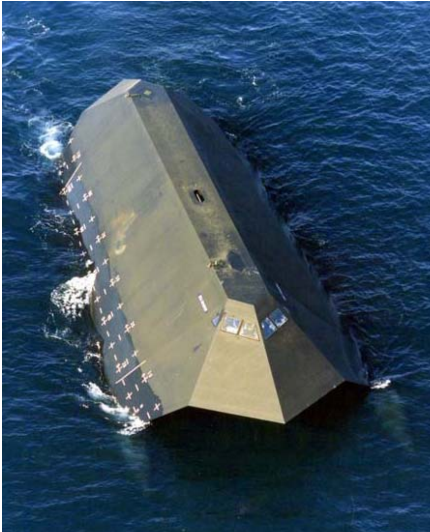
Figure 54: Sea Shadow Stealth Ship Used Radar Deflecting Technology Used in the F-117 Nighthawk Stealth Fighter
