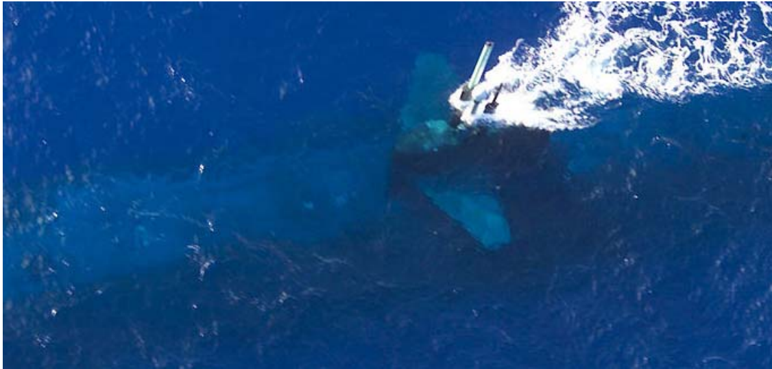
Figure 75: USS Key West off the Coast of Honolulu, Hawaii with masts and Antennae Raised at Periscope Depth
