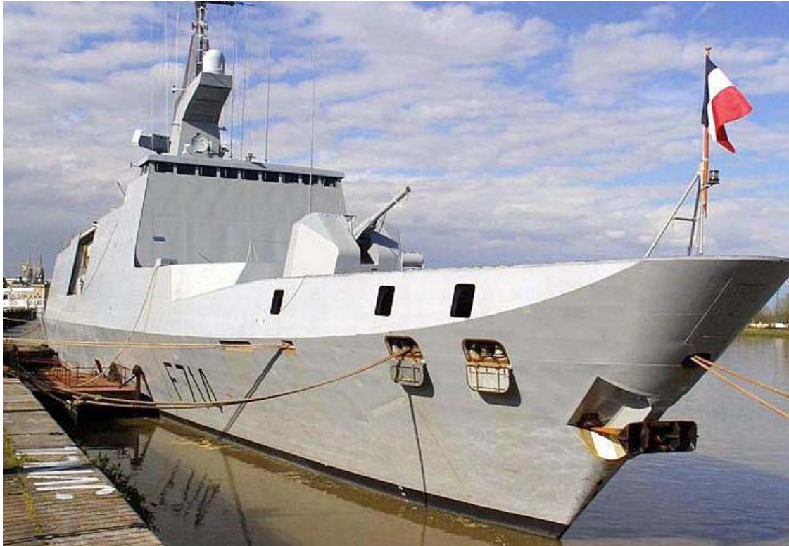
Figure 57: Stealth Radar Deflecting Technology Implemented into a French Lafayette Class Frigate, 2001
