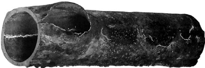
Figure 7.2 Typical furnace waterwall tube overheat failure. ( Babcock & Wilcox, a McDermott company. )
