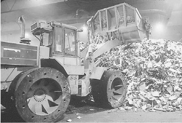
Figure 13.18 Front-end loader moves MSW from tipping floor to processing lines. ( National Ecology, a Babcock & Wilcox company. )
