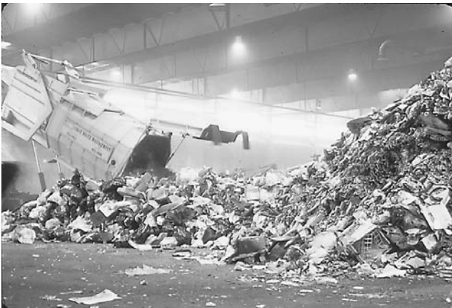
Figure 13.17 Truck dumping MSW onto tipping floor. ( National Ecology, a Babcock & Wilcox company. )
