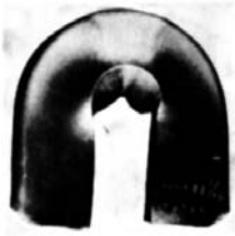
Figure 3.7 Bend-test specimen with the outside fibers elongated 55 percent. ( Babcock & Wilcox, a McDermott company. )
