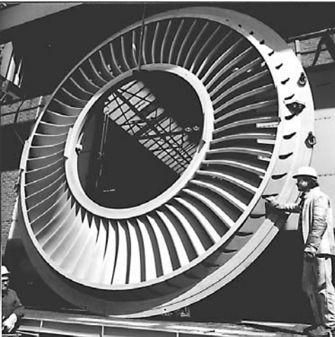
Figure 9.24 Forward-curved last-stage stationary blades. ( Siemens Westinghouse Power Corp. )
