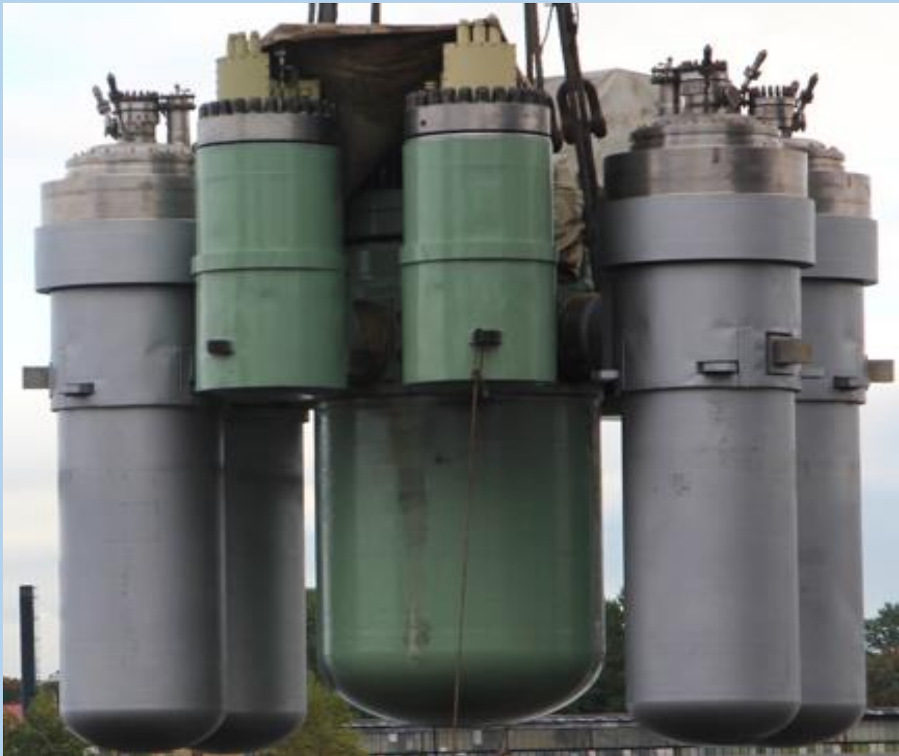
Reactor KLT-40S (in the center) with four steam generators (larger cylinders) and four reactor-coolant circulation pumps (smaller cylinders)
