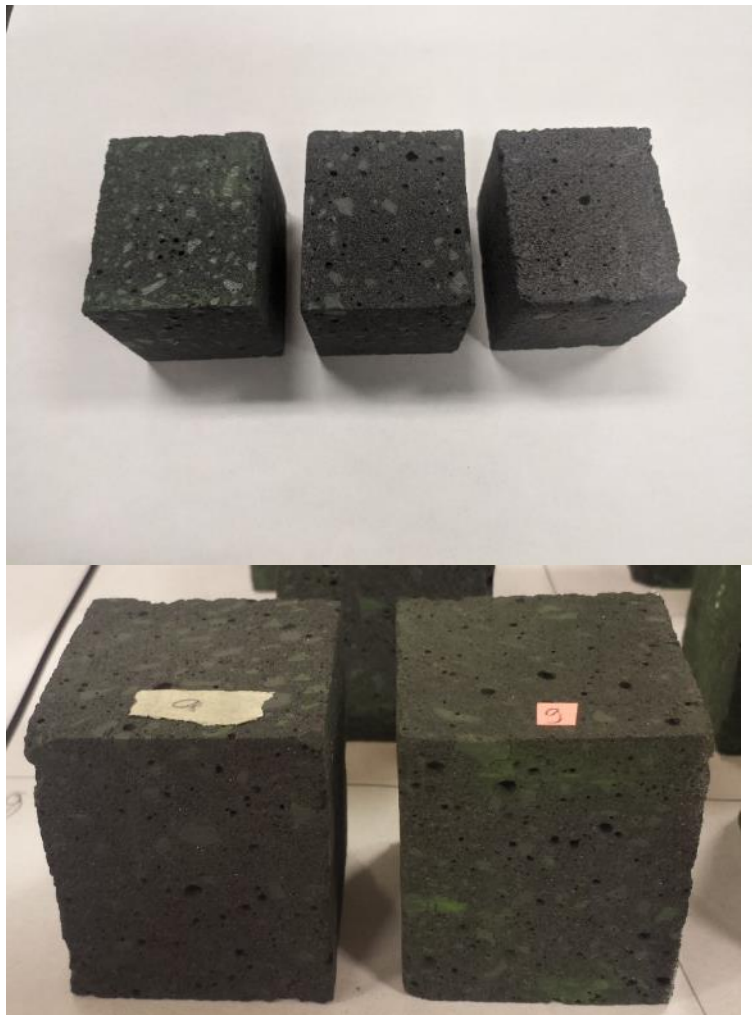
Figure 33: Evolution of brick appearance with thermal cycling.
