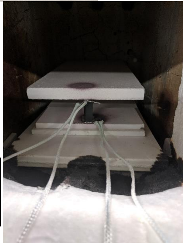
Figure 27: Bulk and contact resistivity-temperature measurement setup for lab-fabricated samples. Two additional platinum leads were run into the furnace chamber to measure voltage as close as possible to the sample.
