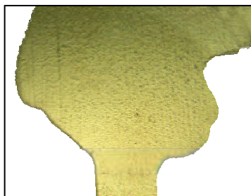
FIG. 27. Slight oxidation film
