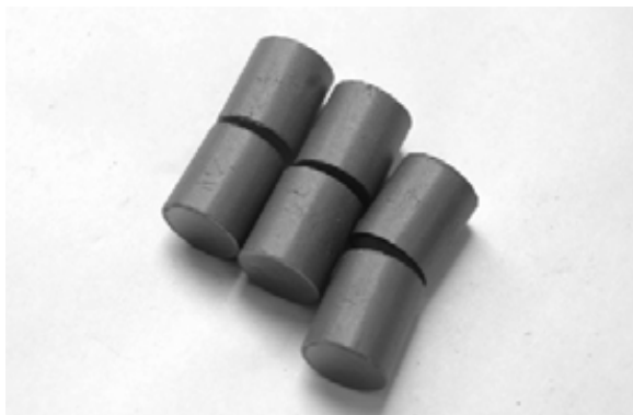
FIG. 21. Typical visual cracks on sintered pellets.
