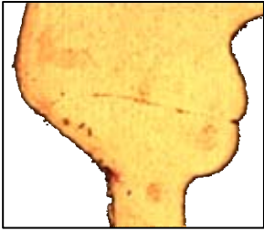
FIG. 12. Discontinuous welding lines in the welding joint
