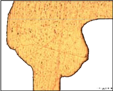
FIG. 13. A continuous thin welding line in the welding joint
