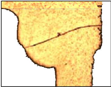
FIG. 14. A continuous thick welding line in the welding joint
