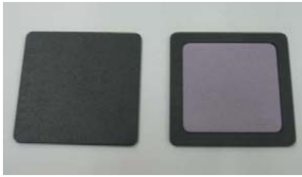
FIG. 4. Erbia-coated graphite plate.
