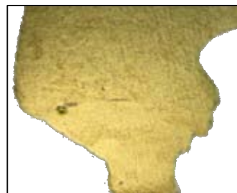
FIG. 28. Serious oxidation film
