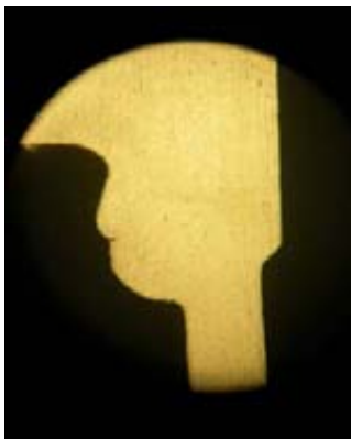
FIG. 5. Welding joint metallographic section
