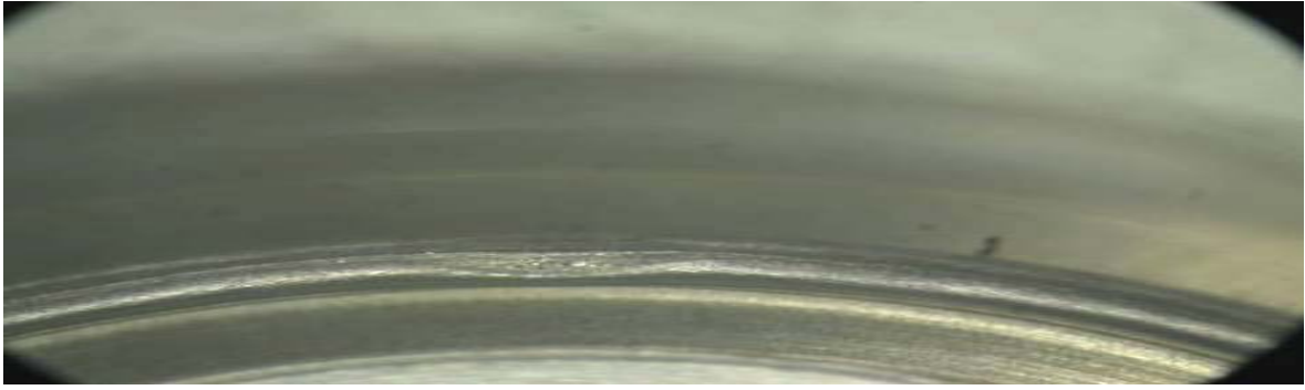
FIG. 18. Photo of the inner upset indentation
