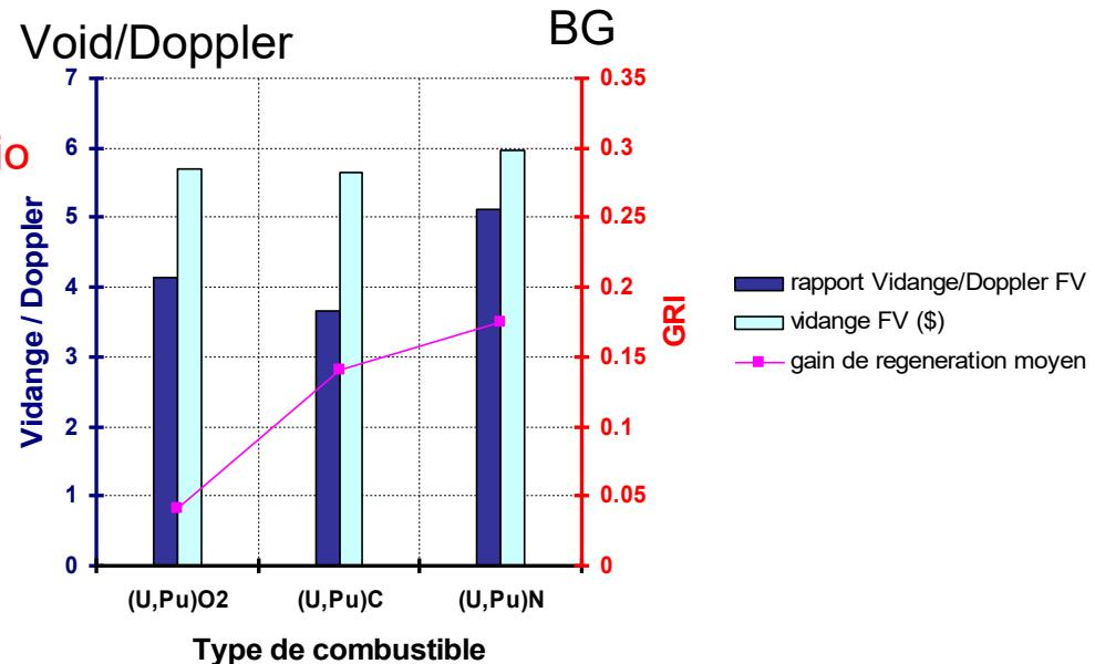
There is a good prospect for enhancement of carbide core features by enhancement of the fuel vol fraction vs sodium, that will yield better BR (more U8) and reduce void worth (less Na). That is made possible due to good thermal properties of carbide Alternatively potential for increasing Pvol, or designing a core with more neutrons leakage
