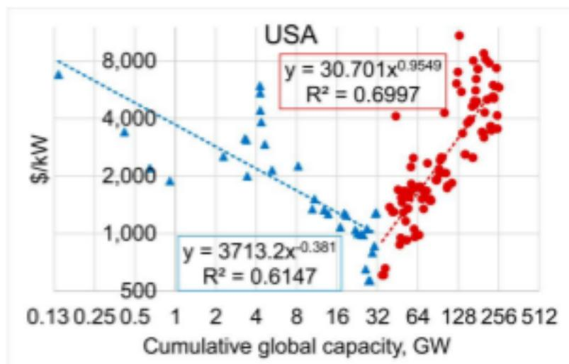
Figure 7.11: USA Unit cost versus capacity [from Lang-2017]
