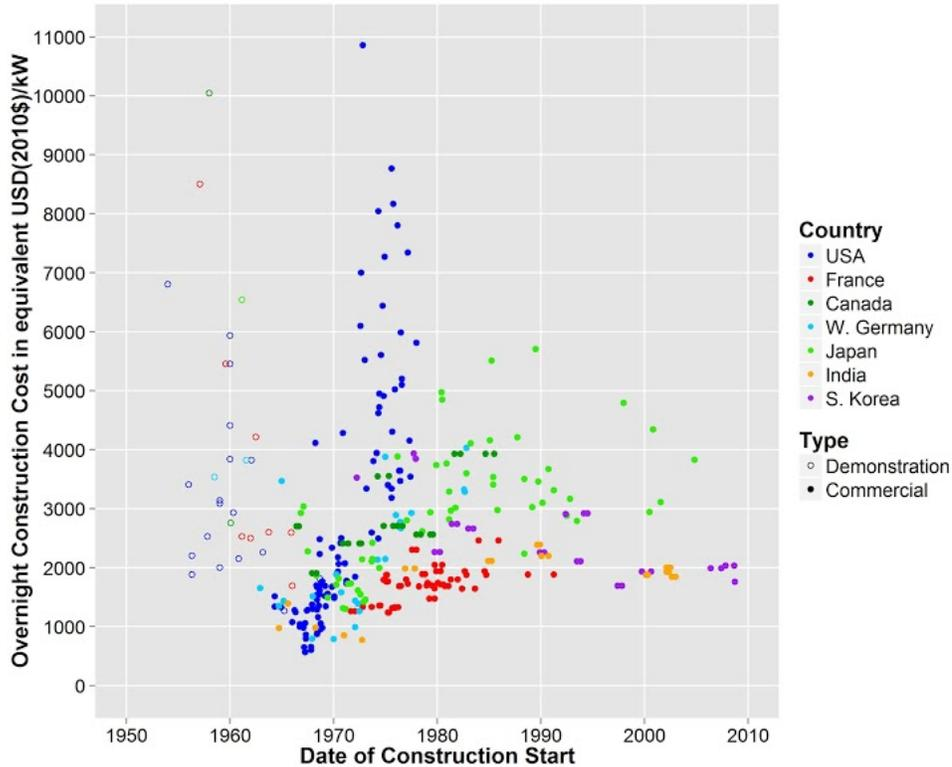
Figure 7.10: Overnight nuclear plant cost as a function of start of construction from [100]
