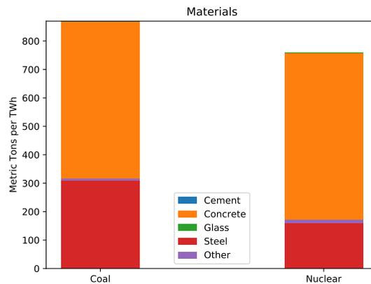
Figure 7.4: Concrete and steel, coal versus nuclear.[128][Table 10.4]
